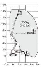
A13JE-Li Working Range 4m 2m 0 STD-1 2m **M** 4m -2m 0 2m 4m 6m 8m
